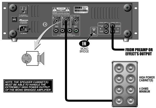
Set the Stereo/Dual Mono / Mono Bridge switch to the Mono Bridgel position (switch in/depressed). Connect a shielded signal cable from the Output of your Preamp or Effect to the Power Amp A Power Amp Input jack. Connect a speaker cable from the SVP1600's Mono Bridge Speaker Output jack to the input jack(s) of the speaker(s). **NOTE: The Speakon® cable must be wired as follows: 1+ = hot, 2+ = return.**
